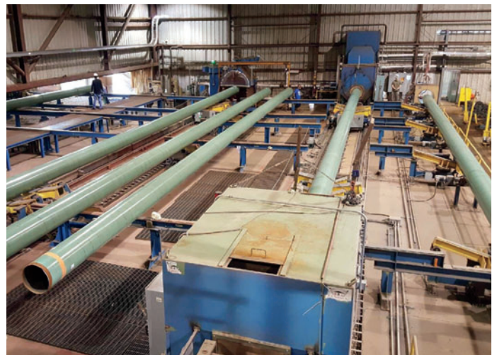
New 12" - 24" diameter pipe coating line at Birmingham, AL facility provides enhanced flow efficiency to oil and gas pipelines.
