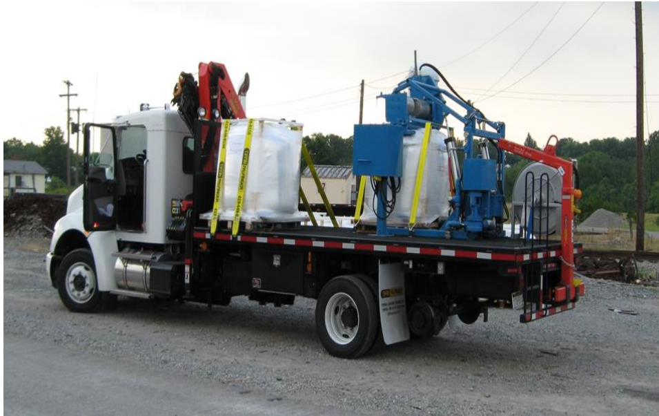
Bulk Filling Truck with Knuckle Boom Crane and Squeezer System
