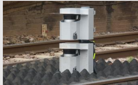
LIDAR used to Detect Debris at Crossings
