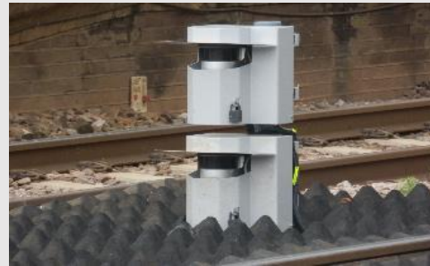
LIDAR used to Detect Debris at Crossings
