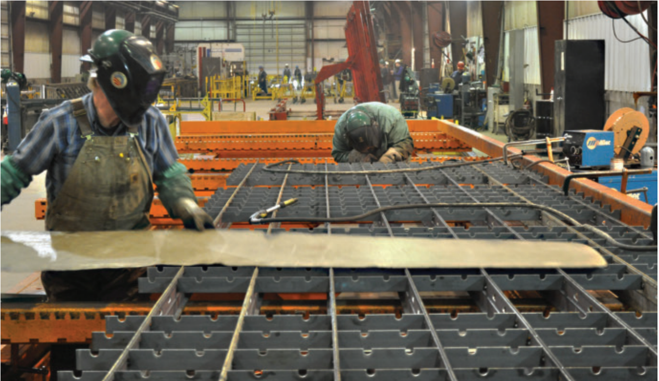
Skilled team at Fabricated Bridge Products plant in Bedford, PA manufacturing reliable steel grid decking for use on North America's most important spans.
